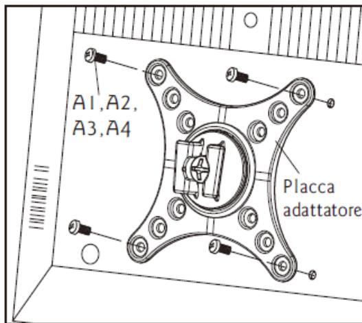
Per fissare le viti M4 e M5 allo schermo.
