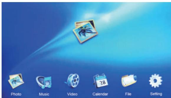
In main menu you can select the storage to display by pressing **EXIT**. Only detected storage will be selectable (by using ◀ ▶ keys) and confirm with **ENTER**.
